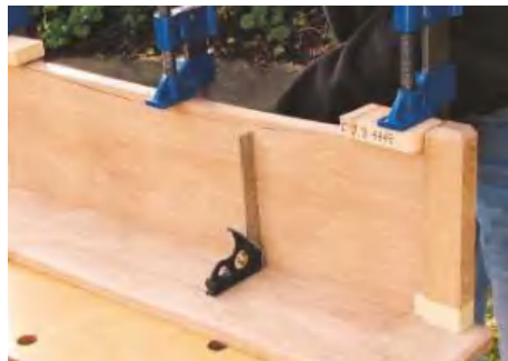
STEP 14. Glue the rear panel and shelf together, checking for square as you tighten the clamps
